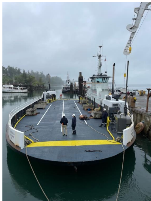
Ferry undergoing the incline test.
